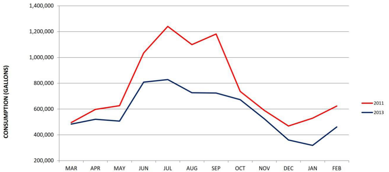
AT&T City Center, Birmingham, AL 2000-tons Cooling WATER USE COMPARISON 30-Story Office Building
