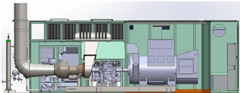
*Above picture represents component parts of Turbine system inside container*
