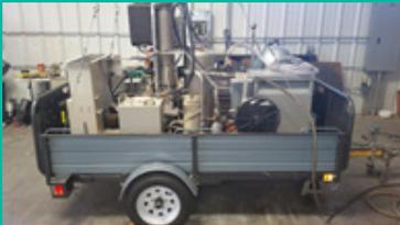
*Picture of HYDROSYNE Fuel System that supplies approximately 500 liters per minute of fuel*
